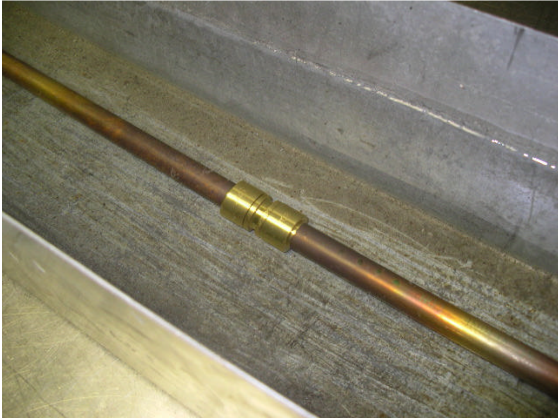
Figure 5 Specimen 04-044-5-1, submerged in water bath, post fire exposure
